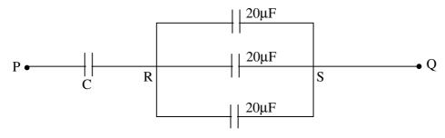
Calculate the capacitance of the capacitor C in diagram. The equivalent capacitance of the combination between P and Q is 30  $\mu F$ .
